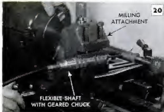
Accurate cross drilling can be done with flexible shaft held in milling attachment. Latate centers accurately
